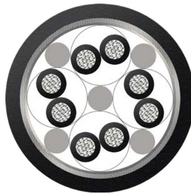
BizLink Sealine® BWTS cable 4x2x0.75 VZN BK 订购号: L45551-D42-K16
