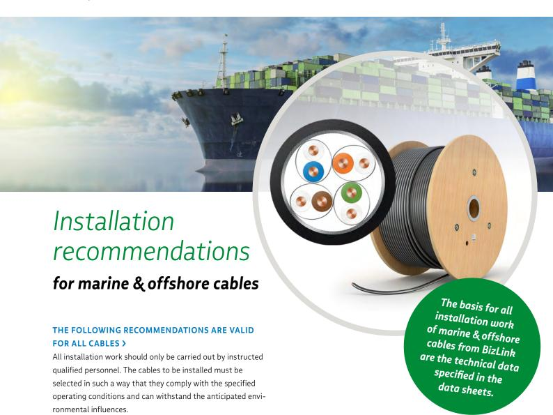
The installation work should only be carried out with cables at a uniform temperature, observing the minimum laying temperature.
