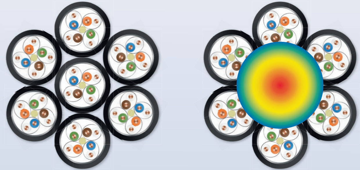
Example of application for an Ethernet cable bundle with PoE use with resulting heat generation
